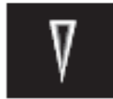
Warning of 'Give way' line
