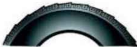
Diagonal Wear/ Heel and Toe Wear
