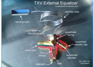
evaporator and the pressure of the evaporator, the TXV can control the gas leaving the evaporator at a predetermined superheat.
