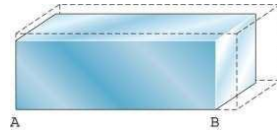
FIG. 2-19 Block of material subjected to an increase in temperature
