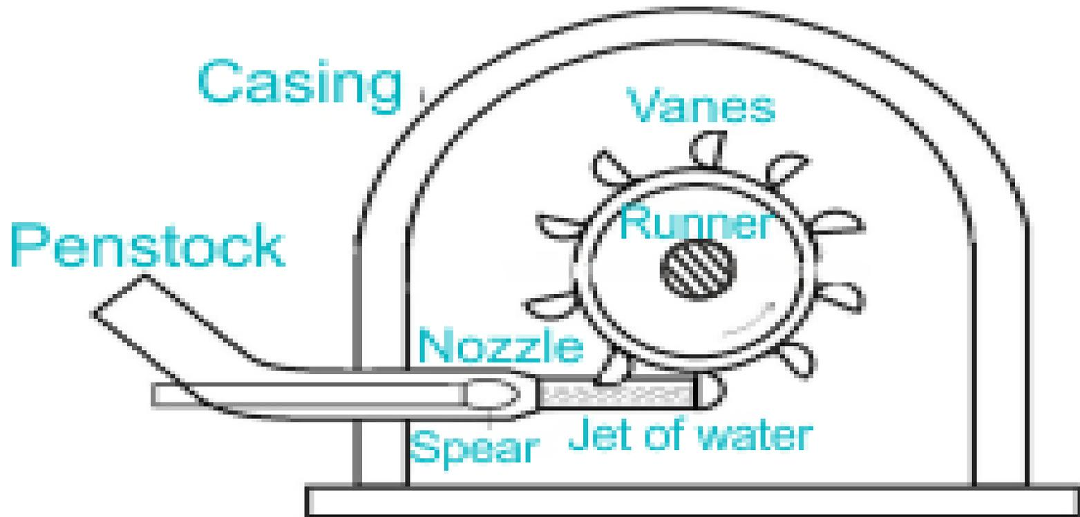
**Pelton Wheel Turbine Line Diagram**
