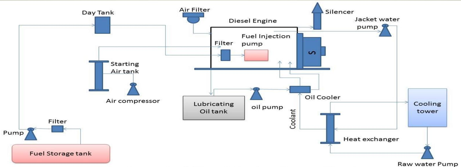
Layout of Diesel Engine Power Plant
