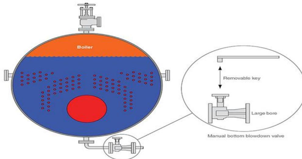
Fig. 3.14.2 Bottom blowdown valve with removable key
