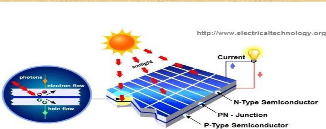
**Basic Operating Principle of a Solar Cell**
