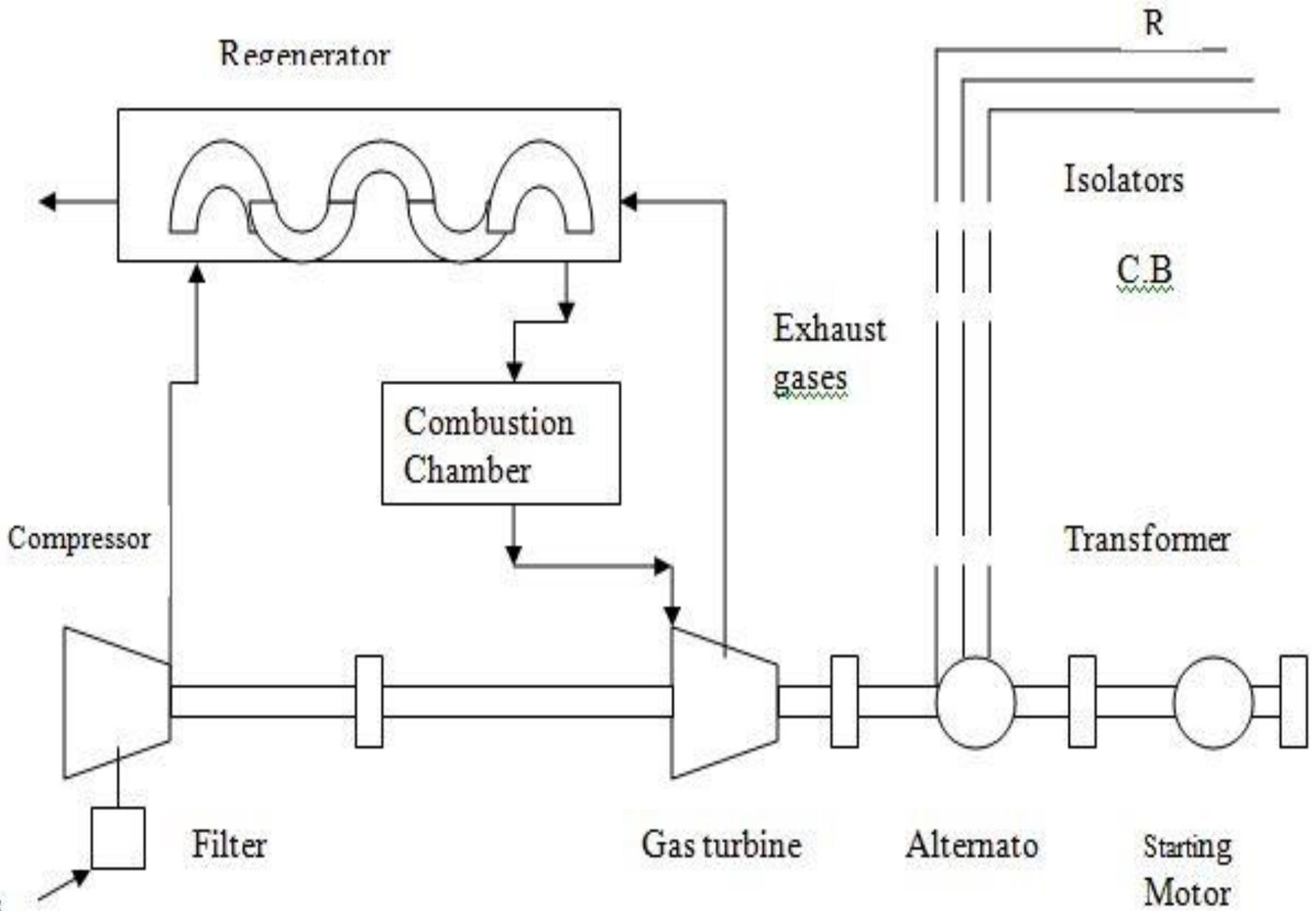
a Schematic arrangement of Gas Turbine Power Station
