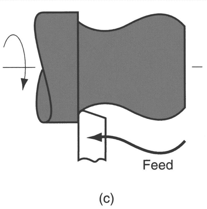
Instead of feeding the tool parallel to the axis of rotation, tool follows a contour that is not necessarily straight (thus creating a contoured form).
