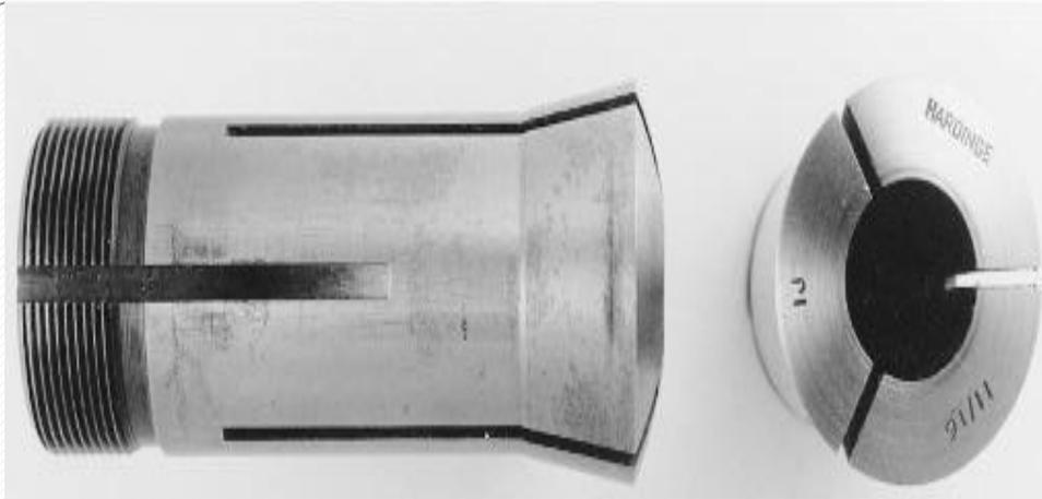
Collet chuck is used to hold small workpieces
