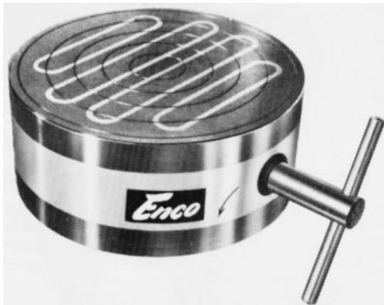
Thin jobs can be held by means of magnetic chucks.
