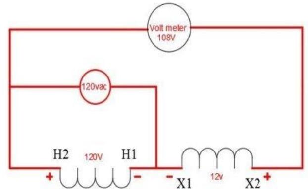
Test- Subtractive Polarity
