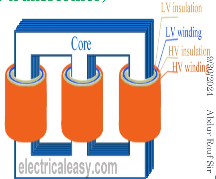
Core type three phase transformer
